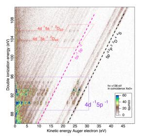
Fig. 8 2D map of core valence double photoionization of Xe atoms at 136 eV photon energy presenting the energy of the double ionized states  $h\nu - (E_1 + E_2)$  against the energy  $E_3$  of the third (Auger) electron.
