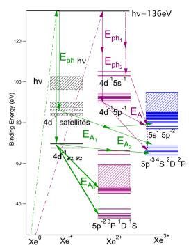
Level diagram of the energy levels relevant for the interpretation of Fia. 7 Fig. 8.
