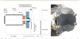
Fig. 2 Schematic of the new magnetic bottle design and ion time-offlight setup. (left) a photo of the cross-shaped magnet assembly with a hole diameter of 4 mm.
