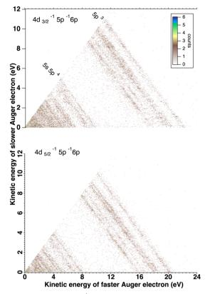
Fig. 6 Decay of xenon 4d5p<sup>-1</sup> 6p shake states by emission of two Auger electrons. The three electrons are detected in coincidence with Xe<sup>3+</sup> ion. The 2D plot of the Auger double electrons are filtered according the satellites photoelectron lines  $\sim$  49 eV (top) and  $\sim$  51 eV (bottom).
