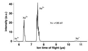
Fig. 4 Ion time-of-flight showing the production of  $Xe^{q+}$  ions  $(q \le 4)$ .
