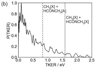
Fig. 7 Total kinetic energy release (TKER) distribution for the (a) N-CO and (b) N-CH<sub>3</sub> bond fission channels following 245 nm photolysis of DMF. The total available energies for the possible product channels are indicated by dashed vertical lines.
