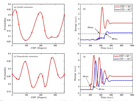
Fig. 4 (a) CEP-dependent single dissociative ionization channel probability in the case of parallel orientation. (b) The single particle energy of the ionized electron for CEP = 30° and CEP = 90° for the parallel orientation. (c) and (d) Same as (a) and (b), but for the perpendicular orientation. The arrows in (b) and (d) indicate the ionization time of the first ionization step. The peak intensity of the laser pulse is  $1 \times 10^{15}$  W cm<sup>-2</sup>.
