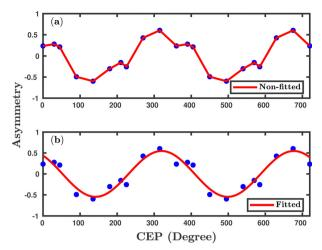
Fig. 8 The asymmetry parameter to elucidate the effect of CEP. The initial orientation of the molecule is parallel to the laser polarization plane. The peak intensity of the laser pulse is  $1 \times 10^{15}$  W cm<sup>-2</sup>. (a) shows non-fitted data and (b) shows fitted data.
