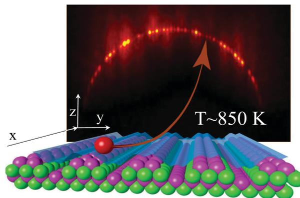
**Fig. 1** Schematic view of a GIFAD setup, the well-aligned row of atoms acts as a grating for the projectile atomic wave. A detector located almost a meter downstream records the diffraction image. The one here, taken from ref. 6 was recorded directly in a MBE vessel with 400 eV He at  $0.65^\circ$  on a GaAs(001) surface at  $\sim 850$  K. The bright spots corresponding to elastic diffraction are located on the Laue circle of energy conservation.
