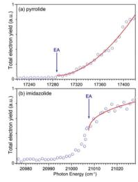
Fig. 6 Photodetachment spectra of (a) pyrrolide and (b) imidazolide. The EA of each anion is indicated by the arrow. The photodetachment spectra are fitted by the Wigner threshold law:  $\sigma = A \times (h\nu - EA)^{l+1/2}$ , where A is the parameter related to the PE signal intensity,  $h \nu$  is the photon energy, and lis the angular momentum of the photoelectron. The *l* value is found to be 1.4 for (a) and -0.1 for (b).
