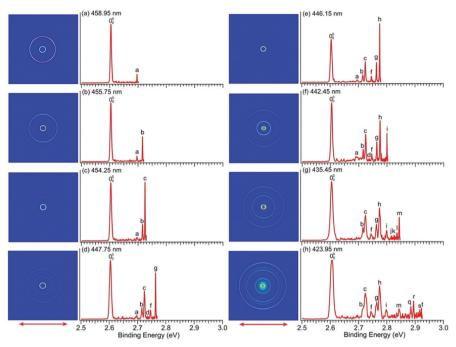
Fig. 5 PE images and spectra of the imidazolide anion at (a) 458.95 nm (2.7015 eV), (b) 455.75 nm (2.7204 eV), (c) 454.25 nm (2.7294 eV), (d) 447.75 nm (2.7691 eV), (e) 446.15 nm (2.7790 eV), (f) 442.45 nm (2.8022 eV), (g) 435.45 nm (2.8473 eV) and (h) 423.95 nm (2.9245 eV). The double arrows indicate the polarization direction of the detachment laser.
