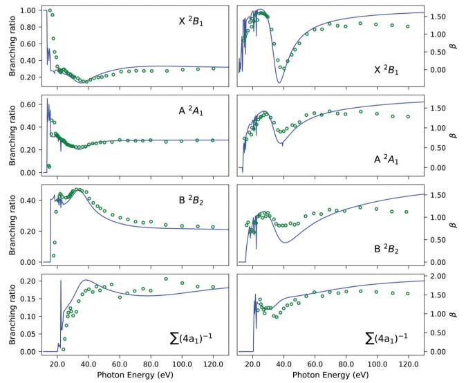
Fig. 5  $H_2$ S. Branching ratio (left panels) and asymmetry parameter  $\beta$  (right panels) obtained using the EOM-CC3/aug-cc-pVTZ Dyson orbital description of the bound state with the B-spline TD-DFT continuum (solid blue line) *versus* experiment (green circles). The summation in the bottom panels refers to the four  $4a_1$  states listed in Table 3. The experimental results were re-digitized from ref. 94.
