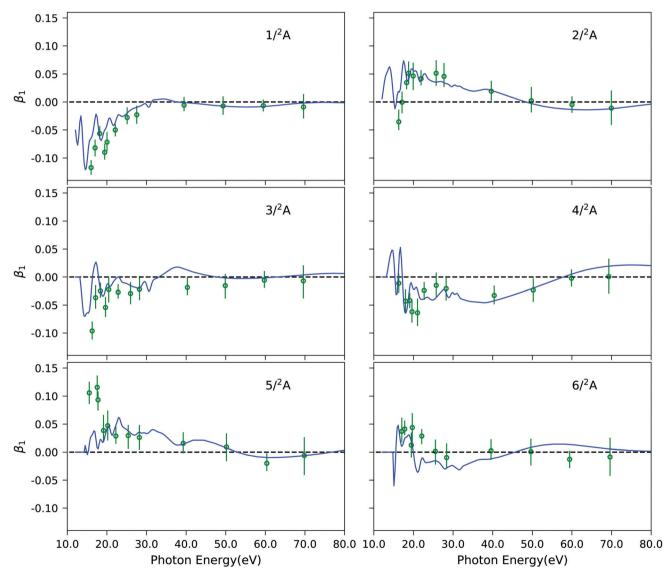
Fig. 7  $C_3H_6O$ : photoelectron circular dichroic parameter  $\beta_1$  computed using EOM-CC3/aug-cc-pVTZ Dyson orbitals and B-spline TD-DFT continuum orbitals, shown by blue lines. Experimental results (green dots) were taken from ref. 97. The spectral features are convoluted using Gaussian broadening of full width at half maximum of 1.0 eV.
