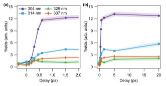
Fig. 2 Experimental results of yields of dissociating molecules in (D+, D+, CO+) channel at each wavelength as a function of pump-probe time delay (a) between -0.3 ps to 2 ps and (b) up to 20 ps. Hatched areas denote the statistical errors.
