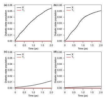
Fig. 3  $\tilde{X}$  and  $\tilde{T}_1$  diabatic state populations within 2 ps calculated following the selective population of the out-of-plane bending (Q<sub>4</sub>) and C-O stretching  $(Q_2)$  modes in the  $\tilde{A}$  state. (a)  $Q_2^4 Q_4^1$  (304 nm), (b)  $Q_2^3 Q_4^1$ (314 nm), (c)  $Q_2^2 Q_4^1$  (329 nm), (d)  $Q_2^1 Q_4^1$  (337 nm).
