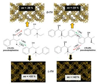
**Fig. 1** Scheme of the synthetic route to the two enantiomorphic crystal-line polymorphs of the **-ITV** framework ( $P4_132$  and  $P4_332$  space groups) by using the two derivatives of the enantiomers of pseudoephedrine through GTM-3 (by attachment of an ethyl group, red-arrows routes) or GTM-4 (by attachment of a benzyl group, green-arrows routes). D/L notation is arbitrary and does not mean an actual absolute configuration of the zeolite.
