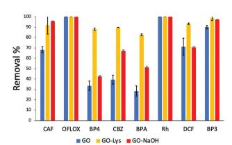
**Fig. 2** Removal of EC mix (5 ppm each,  $V_{\rm tot} = 25~{\rm mL}^{-1}$ , 25 mg of sorbent, contact time 24 h (data at 1 h and 4 h are reported in Fig. S7 and S8 ESI†). The acronyms refer to the molecules shown in Fig. S1, ESI.†
