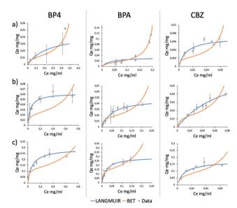
**Fig. 4** Adsorption isotherms of GO (a), GO-NaOH (b) and GO-Lys (c) for BP4, BPA and CBZ (from left to right). Blue lines, Langmuir model; red lines, BET model.
