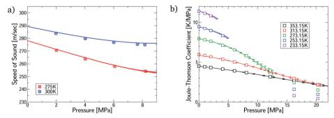
Fig. 3 Comparison of the first-principles predictions for CO<sub>2</sub>-Ar mixtures via our virial calculations. (a) Speed of sound measurements<sup>32</sup> at  $\phi_{\text{CO2}} = 0.5$ ; and (b) Joule-Thomson coefficient measurements<sup>33</sup> at  $\phi_{CO2} = 0.464$ . All predictions are converged with respect to number of virial terms.
