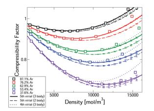
Fig. 2 Comparison of the first-principles predictions of the compressibility factor of CO<sub>2</sub>-Ar mixtures at 323.15 K and measurements.<sup>31</sup>
