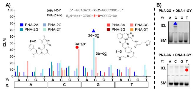
Fig. 4 (A) ICL% of PNA-2 (a) and PNA-3 (b) series towards DNA-1-XY. Experiment performed in PBS buffer, pH 7.4 (100 mM NaCl, 10 mM phosphate), at 5 µM strand concentration, upon addition of 4.0 equivalents of NBS. The experiment leading to a confirmed ICL formation are indicated in the graph (2G-GC, 3A-CT, 3A-GC). (B) Examples of PAGE analysis for PNA-2G + DNA-1G-Y and PNA-3A + DNA-1Y. The reacting nucleobases are underlined. Experiments were performed as single replicates.
