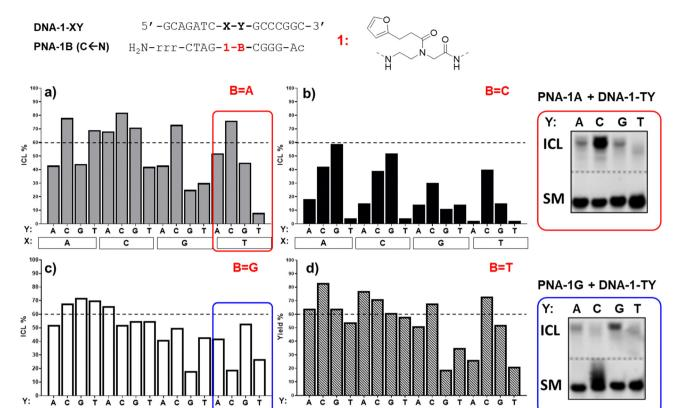
Fig. 3 ICL yield (%) of PNA-1 series equipped with 1, towards DNA-1-XY (X = nucleobase facing 1; Y = nucleobase facing B), and representative PAGE analysis examples. (a) ICL% of PNA-1A. (b) ICL% of PNA-1C. (c) ICL% of PNA-1G. (d) ICL% of PNA-1T. The dashed line indicates the 60% yield threshold. Experiment performed in PBS buffer, pH 7.4 (100 mM NaCl, 10 mM phosphate), at 5 μM strand concentration, upon addition of 4.0 equivalents of NBS. Experiments were performed as single replicates.
