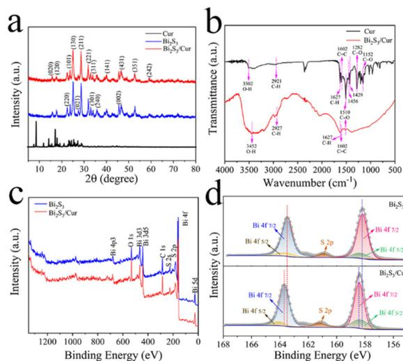
**Fig. 2** (a) XRD patterns of Cur, Bi<sub>2</sub>S<sub>3</sub> and Bi<sub>2</sub>S<sub>3</sub>/Cur. (b) FTIR spectra of Cur and Bi<sub>2</sub>S<sub>3</sub>/Cur. (c) XPS spectra of Bi<sub>2</sub>S<sub>3</sub> and Bi<sub>2</sub>S<sub>3</sub>/Cur. (d) XPS spectrum of Bi 4f.
