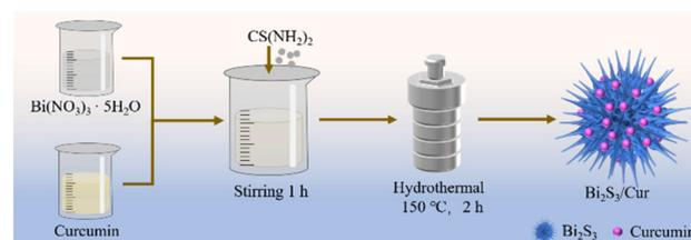
**Scheme 2** Schematic diagram of  $\text{Bi}_2\text{S}_3/\text{Cur}$  hybrid material synthesis.
