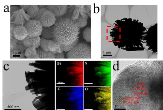
**Fig. 1** Morphology and microstructure of as-synthesized materials. (a) SEM image of Bi<sub>2</sub>S<sub>3</sub>/Cur. Scale bar: 1 μm. (b and c) TEM and element mapping of Bi<sub>2</sub>S<sub>3</sub>/Cur, scale bar: 1 μm, 500 nm. (d) HRTEM, scale bar: 10 nm.
