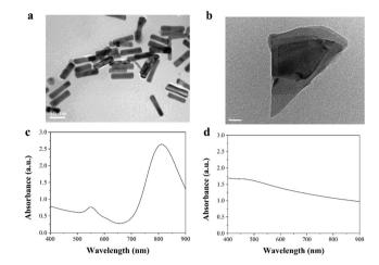
Fig. 1 Characterization of AuNRs and BPNSs. Transmission electron microscopy images of (a) AuNRs and (b) BPNSs. UV-vis spectra of (c) AuNRs and (d) BPNSs.
