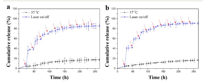
Fig. 4 Release profiles of Dox from (a) Dox-lipo/Au/Gel/PGA and (b) Dox-lipo/BP/Au/Gel/PGA composite scaffolds in PBS at a constant temperature of 37 °C and during a periodic on/off of 1.6 W cm<sup>-2</sup> NIR laser irradiation for 10 min. The arrows indicate the time point when the NIR laser irradiation started. Data are presented as the means  $\pm$  S.D (n = 3).
