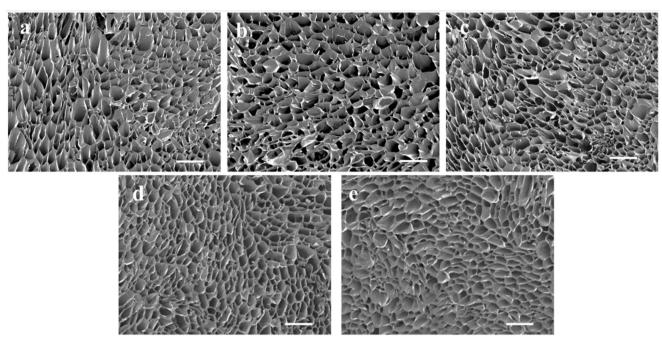
Fig. 2 Scanning electron microscopy images of (a) Gel/PGA, (b) Au/Gel/PGA, (c) BP/Au/Gel/PGA, (d) Dox-lipo/Au/Gel/PGA and (e) Dox-lipo/BP/Au/ Gel/PGA composite scaffolds. Scale bar: 500  $\mu m$ .
