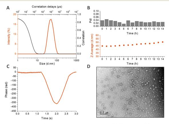
Fig. 6 Physicochemical characterization of the self-assembled nanoparticles based on HA<sub>4,6k</sub>-ELPn80 bioconjugates. (A) Size distribution (in intensity) and correlogram from DLS analysis at 50 °C (78 µM in PBS). (B) Stability over time at 37 °C: evolution of the Z-Average and the PdI measured by DLS with time (78 µM in PBS). (C) Zeta potential measurements (78 µM in HEPES buffer, 60 °C). (D) TEM micrograph (2.6 µM in pure water, drop deposition at 80 °C, and samarium acetate staining).
