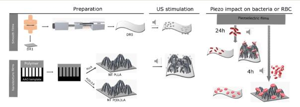
Fig. 1 Schematic presentation of the preparation of smooth piezoelectric (DR5) and non-piezoelectric (DR1) and nanotextured piezoelectric (NT PLLA) and non-piezoelectric (NT P(DL)LA) polymer films and their expected response to ultrasound stimuli as generation of positive charge on the stretched upper side of the down bent polymer and negative charge on the bottom bent side; and piezo-stimulated damaging impact on bacteria for nanotextured film and not harmful behaviour towards RBCs.
