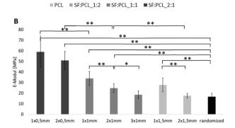
Fig. 5 (A) Elastic moduli of PCL and SF-PCL specimens with varying spinning distance, a voltage of 20 kV and 10% concentration, dotted lines indicate the range of native TM specimens (~20-60 MPa), missing graphs indicate no spinability of the missing case group; (B) influence of oriented fibers spun with varying gap widths and number on Young's modulus of 10% PCL, 20 kV, 20 cm; \* p < 0.05; \*\* p < 0.01.
