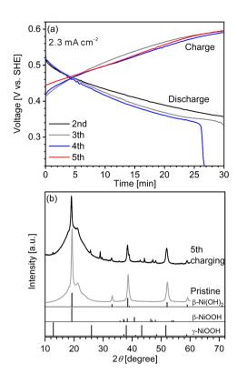
Fig. 2 (a) Charge–discharge curves for the model cathode. (b) XRD patterns of the model cathode after the fifth charging and of the pristine model cathode. The reference peak patterns of  $\beta$ -Ni(OH)<sub>2</sub>,  $\beta$ -NiOOH, and  $\gamma$ -NiOOH are from the powder diffraction file numbers of 00-059-0462, 00-059-0464, and 00-006-0075, respectively.
