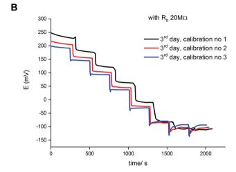
Fig. 4 (A) Selected potentiometric calibration plots for potassiumselective ISE, bypassed by zinc wire and resistor  $R_b = 20 \text{ M}\Omega$ , third calibration for each consecutive day is presented: (1) 1st day. (1) 2nd day (1) 3rd day. (B) Time traces for the sequential calibrations of the 3rd day.
