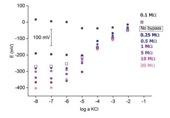
Fig. 2 Potentiometric calibration plots for  $K^+$ -selective ISEs, non-bypassed or bypassed by zinc wire and resistor  $R_{\rm b}$ . Bottom panel: experimental points were shifted to common value for  $\log a$  KCl = -1.
