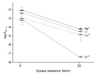
Fig. 5 Effect of applied bypass resistance on the selectivity of potassium-selective ISE, mean value of logarithm of selectivity coefficient + SD is shown, the value presented was determined for activity range from 10<sup>-3</sup> to 0.1 M using experimental slopes.
