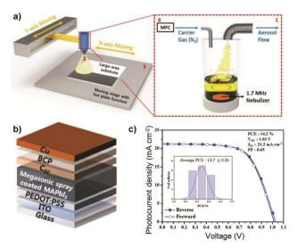
Fig. 4 (a) Schematic representation of the megasonic spray-coating process. (b) Schematic illustration of an inverted planar MAPbI3 perovskite solar cell fabricated via the megasonic spray-coating system. (c) J-Vcurves and histogram (inset) of 18 megasonic sprayed perovskite solar cells with a 1 cm<sup>2</sup> active area under one sun illumination. Reproduced with permission.<sup>85</sup> Copyright 2018, John Wiley and Sons.
