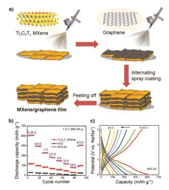
Fig. 3 (a) Schematic representation of the manufacturing of free-standing and flexible 2D MXene/graphene heterostructured films by a spray-assisted LbL process. (b) Rate profiles. (c) Charge–discharge curves of the M/G-20 film at different current rates. Reproduced with permission. <sup>63</sup> Copyright 2019, John Wiley and Sons.
