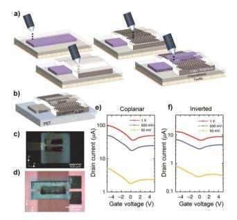
**Fig. 6** (a) Fabrication steps of the inkjet-printed inverted-staggered FET heterostructure on textile. (b) Schematic of a printed inverted-staggered FET heterostructure. (c) Inverted-staggered and (d) coplanar FET heterostructures on PET. (e and f) Transfer characteristics of the FETs as a function of  $V_{\rm ds}$ . Reproduced with permission. Copyright 2017, Springer Nature
