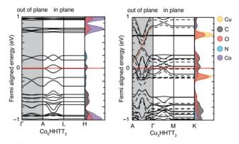
Fig. 2 Electronic band structures of Co-HHTT and Both structures exhibit metallic electronic band structures, shown by the non-zero density of states at the Fermi level (indicated by the red line). The k-points are shown for the in plane and out of plane sections of both two-dimensional structures. Reproduced from ref. 51 with permission from Springer Nature, copyright 2020.
