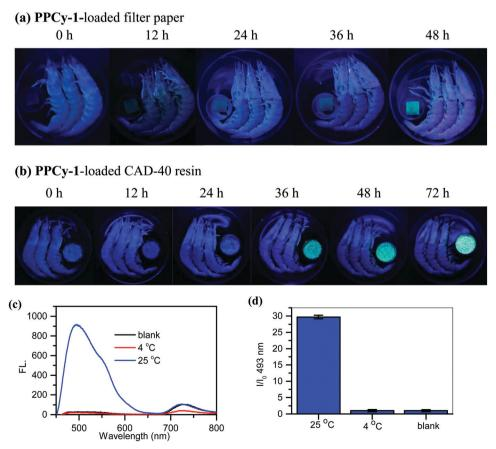
Fig. 8 Monitoring shrimp spoilage at 25 °C by (a) PPCy-1-loaded filter paper and (b) PPCy-1-loaded CAD-40 resin with fluorescent modes. (c) The emission spectra and (d) I/I<sub>0</sub> at 493 nm of the PPCy-1-loaded CAD-40 resin in the absence and presence of shrimp storage at 4 °C and 25 °C for 36 h.
