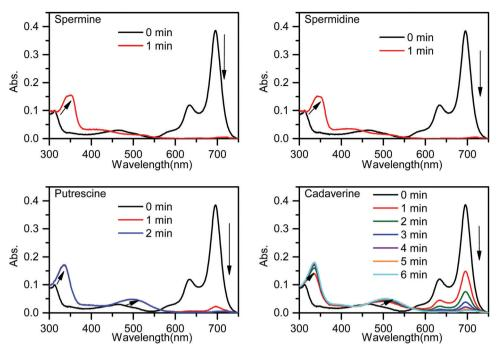
Fig. 1 Time-dependent UV-vis spectra of PPCy-1 (2.5 µM) in the presence of spermine, spermidine, putrescine and cadaverine (50 µM) at room temperature
