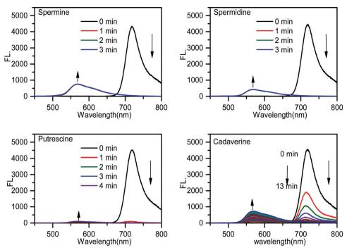
Fig. 2 Time-dependent emission spectra of PPCy-1 (2.5 μM) in the presence of spermine, spermidine, putrescine and cadaverine (50 μM) at room temperature.
