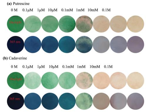
Fig. 6 The color and emission changes of the PPCy-1-loaded filter paper with colorimetric (top) and fluorescent (bottom) dual modes in the presence of (a) putrescine and (b) cadaverine solutions at 25 °C.
