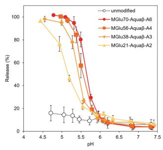
Fig. 3 pH-Sensitivity of liposomes modified with Aquaß derivatives. pH-Dependence of pyranine release from liposomes modified with or without Aguaß derivatives after 30 min incubation are shown. Lipid concentration was  $2.0 \times 10^{-5}$  M. Each point is the mean  $\pm$  SD (n = 3).
