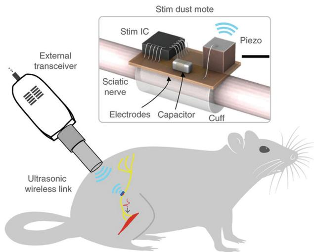
**Fig. 2** Schematic representation of the wireless neural stimulator system is shown here. Piezoceramic transducer is placed on top of the system to receive ultrasonic signals and thus generates electricity. Reproduced with permission. Copyright©2020, Springer Nature.
