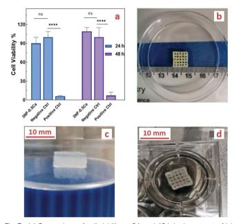
Fig. 7 (a) Comparison of cell viability at 24, and 48 h in the extract of ink 3NF-0.5Ca via SRB assay. (Two-way ANOVA, Sidaks's post-test, p <0.0001.) The lattice-structure printed scaffolds: (b) scaffolds after printing and before photo crosslinking, (c) photo crosslinked scaffolds after swelling in culture media for 48 h, and (d) scaffolds with fibroblasts seeded on top after 1 week in culture media.
