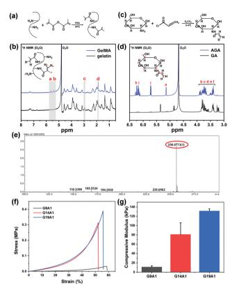
Fig. 1 (a) The synthesis process of gelatin methacrylate (GelMA), (b) <sup>1</sup>H NMR spectra of gelatin before and after modification, (c) the synthesis process of acylated glucosamine (AGA), (d) <sup>1</sup>H NMR spectra of native glucosamine and AGA, (e) mass spectrum of AGA, (f) the stress–strain curves of G9A1, G14A1 and G19A1, and (g) the compressive moduli of G9A1, G14A1 and G19A1.
