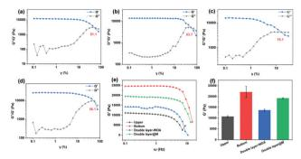
Fig. 3 Shear strain-dependent storage modulus (G') and loss modulus (G'') of (a) upper, (b) bottom, and (c) double-layer hydrogels without chelation, and (d) the double-layer hydrogel after mineralization; (e) storage moduli of the above hydrogels as a function of frequency  $(\omega)$ ; and (f) static moduli of hydrogels collected at a frequency of 1 Hz and 25 °C.
