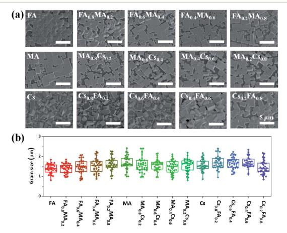
Fig. 3 (a) Top-view SEM images of inkjet-printed  $FA_{1-x}MA_xPbBr_3$ ,  $MA_{1-x}Cs_xPbBr_3$  and  $Cs_{1-x}FA_xPbBr_3$  thin films with x=0, 0.2, 0.4, 0.6, and 0.8, arespectively. (b) Statistical distributions of the grain size of these inkjet-printed films.
