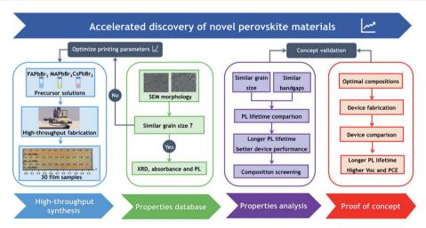
Fig. 1 A framework of our proposed composition screening protocol based on high throughput synthesis.
