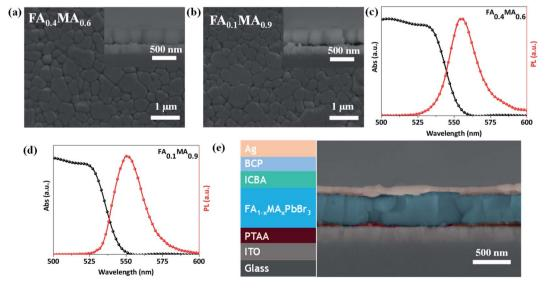
Fig. 5 Top-view and cross-sectional SEM images of spin-coated FA<sub>0.4</sub>MA<sub>0.6</sub> (a) and FA<sub>0.1</sub>MA<sub>0.9</sub> (b) films, respectively. Steady-state PL spectra and absorbance spectra of spin-coated  $FA_{0.4}MA_{0.6}$  (c) and  $FA_{0.1}MA_{0.9}$  (d) films, respectively. (e) Cross-sectional SEM image of a typical cell with a structure of ITO/PTAA/perovskite/ICBA/BCP/Ag.
