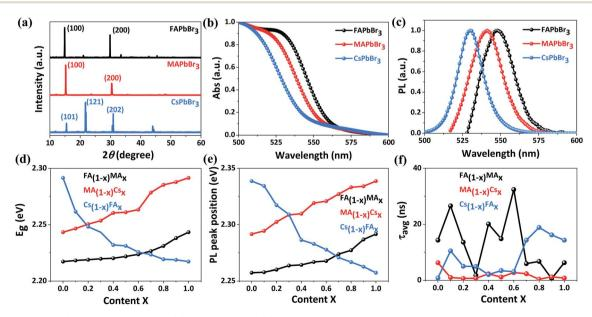
Fig. 4 XRD patterns (a), absorbance spectra (b) and PL spectra (c) of inkjet-printed FAPbBr<sub>3</sub>, MAPbBr<sub>3</sub> and CsPbBr<sub>3</sub> thin films. Bandgaps (d), PL peak positions (e) and average PL lifetimes ( $\tau_{avg}$ ) (f) of inkjet-printed FA<sub>1-x</sub>MA<sub>x</sub>PbBr<sub>3</sub>, MA<sub>1-x</sub>Cs<sub>x</sub>PbBr<sub>3</sub> and Cs<sub>1-x</sub>FA<sub>x</sub>PbBr<sub>3</sub> films as a function of x.
