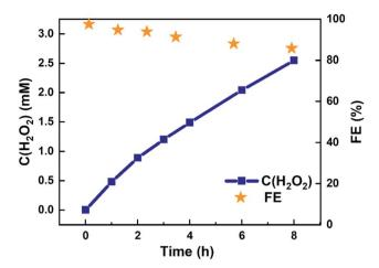
Fig. 3  $H_2O_2$  accumulation using 4:1 (Ti,Mn) $O_x$ -coated FTO electrode operated in the dark. Cumulative  $H_2O_2$  concentration and the respective cumulative FE vs. time. The electrode area was 1.2 cm², and the applied potential was +1.31 V vs. Ag/AgCl (equivalent to an overpotential of 150 mV) in a 20 mL 0.5 M pH = 7.0 PB solution.
