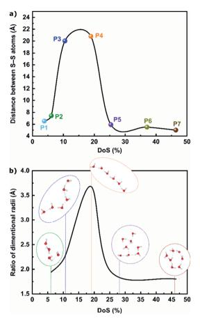
Fig. 5 (a) S-S distance as a function of DoS; and (b) water cluster radii as a function of DoS at 90% RH
