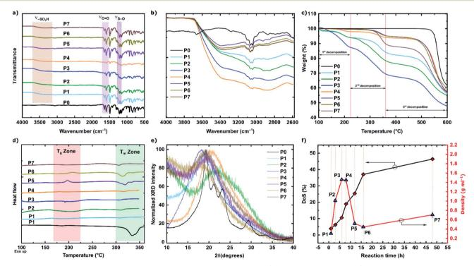
Fig. 2 SPEEK characterization: FTIR spectra in the range of (a)  $500-4000 \text{ cm}^{-1}$  and (b)  $2600-4000 \text{ cm}^{-1}$ ; (c) thermal degradation obtained using TGA; (d) DSC thermograms at  $100-350 \,^{\circ}\text{C}$ ; (e) WAXD spectra with  $2\theta = 8-40 \,^{\circ}$ ; and (f) DoS and densities of polymers as a function of the sulfonation reaction time.
