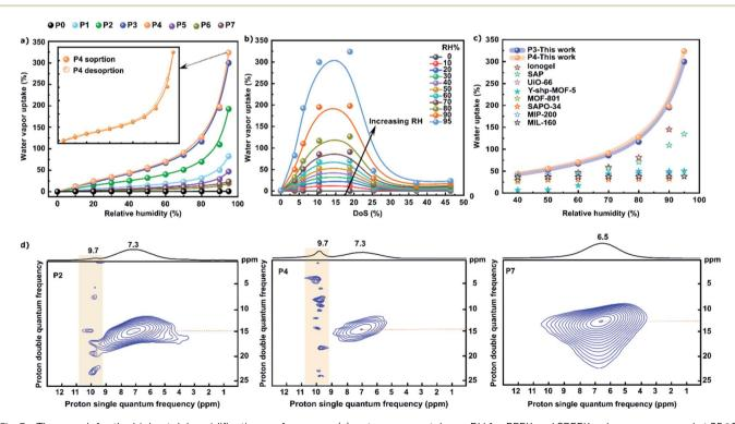
Fig. 3 The search for the highest dehumidification performance: (a) water vapor uptake vs. RH for PEEK and SPEEK polymers measured at 25 °C; hysteresis for P4 is shown in the inset; (b) the effect of DoS on the water vapor uptake; (c) comparison of the performance of P3 and P4 relative to the previously reported materials for water uptake, which are summarized in Table S5, ESI;† and (d) solid state <sup>1</sup>H NMR spectra of P2, P4, and P7 polymers with low, medium, and high DoS, respectively.
