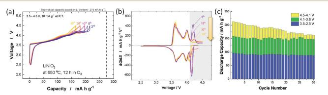
Fig. 1 (a) Galvanostatic charge/discharge curves of LiNiO<sub>2</sub> at a rate of 10 mA  $g^{-1}$ , (b) differential dQ/dE plots obtained from (a), and (c) variations in discharge capacities with different voltage ranges.
