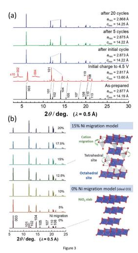
Fig. 3 (a) Synchrotron XRD patterns of LiNiO<sub>2</sub> before and after electrochemical cycles, and (b) simulated XRD patterns with different occupancy of Ni ions at tetrahedral 6c sites. Schematic illustrations of structural models of NiO2 are shown, which were drawn using the program VESTA.20
