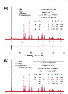
Fig. 4 Comparison of fitting results of Rietveld analysis of the synchrotron XRD pattern of  $\mathrm{Li}_x\mathrm{NiO}_2$  after the 20-cycle test (a) without and (b) with the presence of Ni ions at 6c tetrahedral sites. A clear deviation between simulated and observed patterns for the 101 diffraction line is noted in (a) as marked by the blue arrow.
