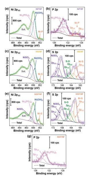
Fig. 3 Ni  $2p_{3/2}$ , P 2p, and S 2p XPS core-level spectra of (a and b) NiP/NF, (c and d) NiS/NF, and (e-g) NiSP/NF samples.
