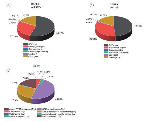
Fig. 3 Breakdown of total capex for a CPV (a) and c-Si PV (b) powered electrolysis process to produce 50 tons  $H_2$  per day using the assumptions listed in Tables 1 and 2. (c) Annual OPEX for both technologies *i.e.* CPV-E and c-Si PV-E.
