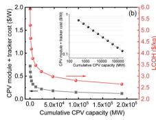
Fig. 4 (a) Module + tracker costs (left) and cost of H<sub>2</sub> (right) as a function of CPV module efficiency (bottom) and STH efficiency (top). (b) Module + tracker costs (left) and cost of H<sub>2</sub> (right) as a function of projected cumulative CPV capacity (bottom). For both projections, the electrolyser efficiency, CAPEX and OPEX were kept constant as mentioned in Tables 2 and 3
