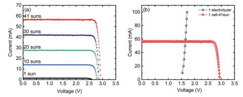
Fig. 1 (a) I-V characteristics of the InGaP/InGaAs/Ge 3J CPV cell (3  $\times$  3 mm<sup>2</sup>) from Azur Space under one sun to 41-sun illumination (note the linearity of the current as a function of light concentration). (b) I-V curve of single alkaline electrolyser (grey) generated using CP measurements overlapped with the I-V curve of the 3J CPV cell (red) under 41 suns (without the use of Fresnel lenses)
