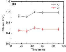
Fig. 2 (a) I-V curves of one (grey) and two 3J CPV cells (red) connected in series under 41-sun illumination overlapped with I-V curves of single (blue) and three (green) alkaline electrolysers connected in series. (b) H2 and O2 production rates from three alkaline electrolysers connected in series. Power is supplied from two CPV 3J cells connected in series under 41-sun illumination (without the use of Fresnel lenses to minimize further losses) as shown in Scheme 1.
