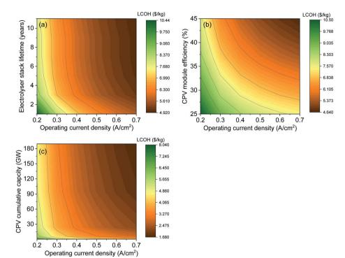
Fig. 5 Contour plots showing the sensitivity of H<sub>2</sub> cost to: (a) electrolyser stack lifetime, (b) CPV module efficiency and (c) CPV cumulative installed capacity versus operating current density of the electrolyser.
