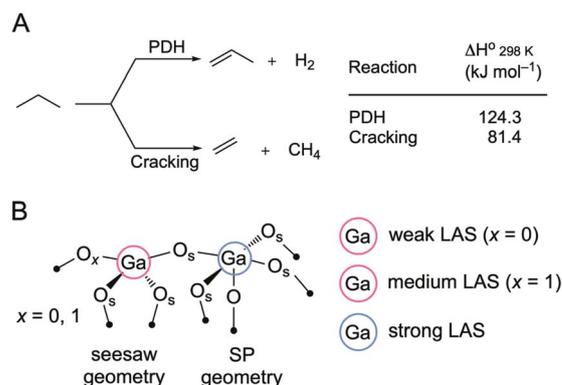
**Scheme 1** (A) Competing propane dehydrogenation (PDH) and propane cracking reactions. (B) A possible coordination geometry for a Ga<sub>IV</sub>-O-Ga<sub>VI</sub> surface linkage with the attribution of Lewis acidity strength according to the <sup>15</sup>N chemical shift of bound pyridine probe molecule.<sup>12</sup> SP stands for square pyramidal.
