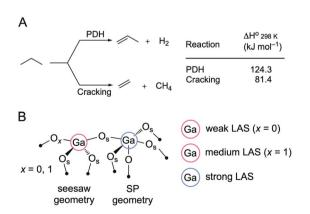
Scheme 1 (A) Competing propane dehydrogenation (PDH) and propane cracking reactions. (B) A possible coordination geometry for a Ga<sub>IV</sub>-O-Ga<sub>VI</sub> surface linkage with the attribution of Lewis acidity strength according to the <sup>15</sup>N chemical shift of bound pyridine probe molecule.12 SP stands for square pyramidal.
