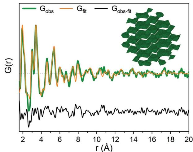
Fig. 8 GaOOH modelled using two GaOOH phases at  $R = 2.5$  for Ga(NO<sub>3</sub>)<sub>3</sub> solution. The refined structure of the large GaOOH phase is shown as the inset.
