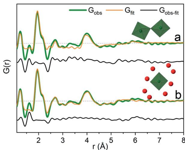
Fig. 3 PDF of the 1 M solution of  $\text{Ga}(\text{NO}_3)_3$  with  $R = 0$  modelled with (a) octahedrally coordinated  $\text{Ga}^{3+}$  in a dimer ( $R_w = 0.412$ ) and (b) a monomer with a second solvent shell ( $R_w = 0.284$ ). The two models are shown as insets with green octahedra representing  $\text{GaO}_6$  and solvent oxygen as red spheres.
