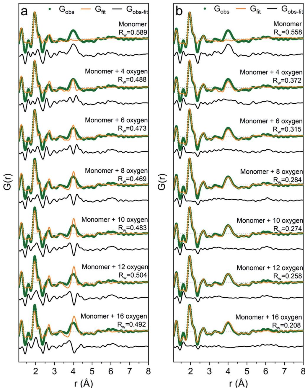
Fig. 5 PDFs of  $\text{Ga}(\text{NO}_3)_3$   $R = 0$  fitted with: (a) the monomer model with different number of solvent oxygen atoms with positions fixed at values in a crystal structure<sup>37</sup> and (b) the same models with refined oxygen positions and a box restraint of  $\pm 0.2$  Å.
