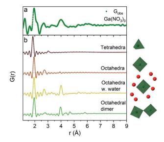
Fig. 2 Comparison of (a) the R=0 Ga(NO<sub>3</sub>)<sub>3</sub> PDF data with (b) calculated PDFs for four small gallium—oxygen structures. From the top the first structure is from the  $\beta$ -Ga<sub>2</sub>O<sub>3</sub> crystal structure,<sup>36</sup> the second and third are from Ga(NO<sub>3</sub>)<sub>3</sub>·9H<sub>2</sub>O<sup>37</sup> and the fourth from the study by Sommer et al.<sup>17</sup>
