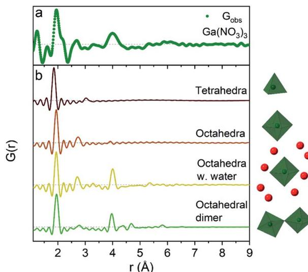
Fig. 2 Comparison of (a) the  $R = 0$   $\text{Ga}(\text{NO}_3)_3$  PDF data with (b) calculated PDFs for four small gallium–oxygen structures. From the top the first structure is from the  $\beta\text{-Ga}_2\text{O}_3$  crystal structure,<sup>36</sup> the second and third are from  $\text{Ga}(\text{NO}_3)_3 \cdot 9\text{H}_2\text{O}$ <sup>37</sup> and the fourth from the study by Sommer *et al.*<sup>17</sup>
