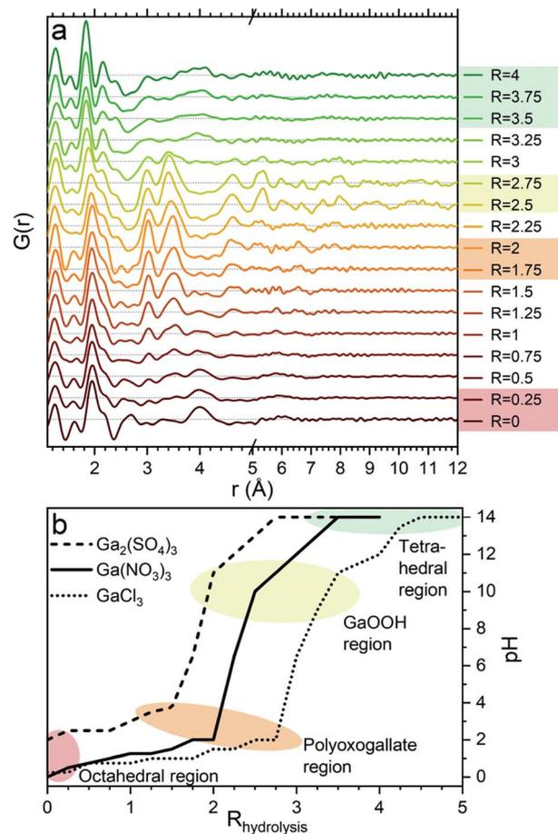
Fig. 1 (a) PDFs of the pH series for  $\text{Ga}(\text{NO}_3)_3$  with increasing hydrolysis ratio,  $R = [\text{OH}^-]/[\text{Ga}^{3+}]$ . The four regions octahedral, polyoxogallate, GaOOH and tetrahedral are marked by colored shading for the data corresponding to similar shaded areas in (b). (b) Measured pH of the three anion series as a function of the amount of added NaOH in the form of the calculated  $R$  showing that the similar structural signals are observed at similar pH.
