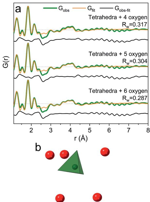
Fig. 9 (a) PDFs of the  $\text{Ga}(\text{NO}_3)_3$  solution with  $R = 4$  modelled with tetrahedrally coordinated  $\text{Ga}^{3+}$  including anions 4, 5 and 6 solvent oxygen atoms. (b) The refined structure with 5 solvent oxygen atoms is shown as the inset with the green tetrahedra representing  $\text{GaO}_4$  and oxygen as red spheres.
