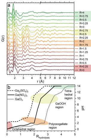
Fig. 1 (a) PDFs of the pH series for  $Ga(NO_3)_3$  with increasing hydrolysis ratio,  $R = [OH^{-}]/[Ga^{3+}]$ . The four regions octahedral, polyoxogallate, GaOOH and tetrahedral are marked by colored shading for the data corresponding to similar shaded areas in (b). (b) Measured pH of the three anion series as a function of the amount of added NaOH in the form of the calculated R showing that the similar structural signals are observed at similar pH.
