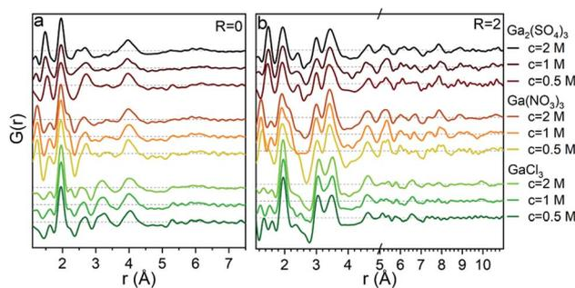
Fig. 11 PDF data for aqueous solutions of  $\text{Ga}(\text{NO}_3)_3$ ,  $\text{GaCl}_3$ , and  $\text{Ga}_2(\text{SO}_4)_3$  with concentrations of 0.5, 1 and 2 M. (a)  $R = 0$  and (b)  $R = 2$ . The variations between the salts is due to differences in pH as outlined in Fig. 1b and Table S12.†
