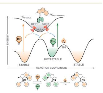
Fig. 7 Simplified potential energy surface (PES) along the isomerisation coordinate, showing the excited state processes occurring during the photochemical E-Z isomerisation. The region of the perpendicular minimum is marked as "dark".
