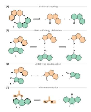
Fig. 12 General synthetic methods for synthesising artificial light-driven molecular motors. (A) McMurry coupling for first-generation overcrowded alkene-based motors; (B) Barton–Kellogg coupling for second- and third-generation overcrowded alkene-based motors; (C) aldol-type condensation chemistry for oxindole-based motors, biomimetic motors, first-generation HTI-based motors; (D) imine condensation for imine-based motors.
