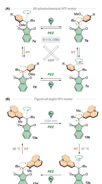
Fig. 4 (A) Rotation cycle of a second-generation hemithioindigobased motor. The single bond rotation (SBR), double bond isomerization (DBI) and hula twist motion (HT) of 7 are highlighted; (B) second-generation hemithioindigo motor 13 with a figure-of-eight rotation cycle.
