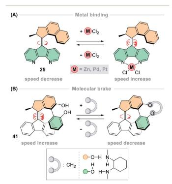
Fig. 11 Modulation of rotation speed of second-generation overcrowded alkene-based motors by allosteric binding. (A) Binding of transition metal ions to the lower half increases the rotation speed; (B) non-covalent binding of molecular tethers to the upper half decreases the rotation speed.
