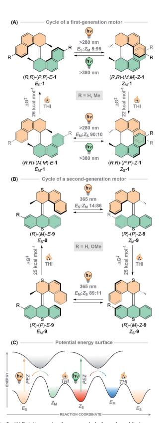
Fig. 2 (A) Rotation cycle of overcrowded alkene-based first-generation motor 1; (B) rotation cycle of overcrowded alkene-based second-generation motor 9; (C) potential energy surface of the rotation cycle of overcrowded alkene-based motors, with photochemical E-Z (PEZ) and thermal helix inversion (THI) steps highlighted.
