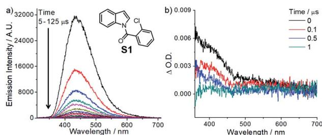
**Fig. 1** (a) Time-resolved emission spectra of **S1** in the solid state (excitation, 355 nm; the arrow indicates the change in emission intensity). (b) ns-TA spectra of **S1** (0.1 M) in degassed MeCN (excitation, 355 nm).
