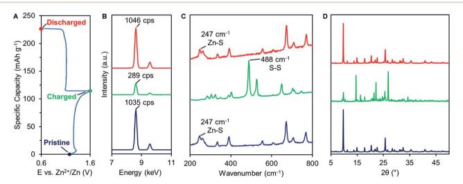
Fig. 4 (A) Typical GCD profile of 2. Ex situ (B) XRF, (C) Raman, and (D) PXRD analysis of pristine (blue), charged (green), and discharged (red) 2.
