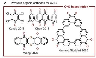
Fig. 1 (A) State-of-the-art organic cathode materials for AZIBs are mostly based on the redox of quinone/phenazine. (B) Zn-thiolate cathode materials reported in this work.
