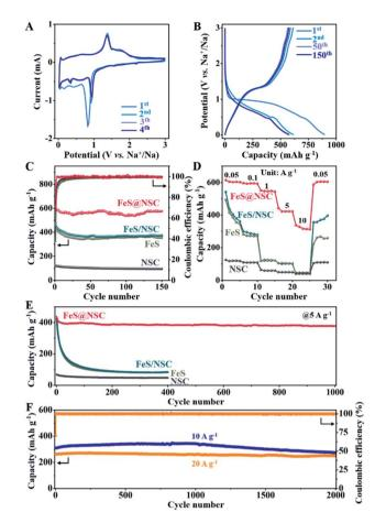
Fig. 4 (A) CV curves of FeS@NSC; (B) charge/discharge curves of FeS@NSC at 0.1 A g $^{-1}$ ; (C) charge capacities and corresponding coulombic efficiencies at 0.1 A g $^{-1}$ ; (D) rate capacities for current densities in the range of 0.05–10 A g $^{-1}$  between 0.01 and 3 V (vs. Na $^+$ / Na); (E) charge capacities of FeS@NSC, FeS, FeS/NSC, and NSC composites at 5 A g $^{-1}$ ; (F) charge capacities of the FeS@NSC composite at 10 and 20 A g $^{-1}$ .
