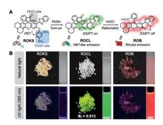
Fig. 3 (A) Our dual-channel fluorescent probe ROKS for sequential and logical identification of PhSH and HOCl, and its reaction scheme. (B) Photographs of ROKS, ROCL and ROB in the solid state and PBS buffer solution (10 mM, pH = 7.4, containing 10% DMF) under natural light and UV light of 365 nm, respectively.
