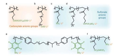
Fig. 3 Anionic groups for constructing SIC polymers. Chemical structures of (a and b) carboxylate-based SIC polymer electrolytes and (c-f) sulfonate-based SIC polymer electrolytes. Black: polymer backbone; olive: anion; orange: Li<sup>+</sup> cation.
