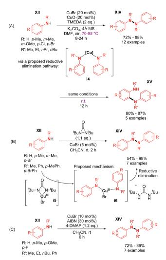
**Scheme 5** Cu-catalyzed N-N dehydrogenative coupling o secondary amines.
