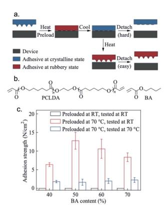
**Fig. 6** (a) Illustration of the transfer process enabled by the adhesive with shape memory microstructure. (b) Chemical structures of PCLDA and BA. (c) Adhesion strength of non-structured samples with different BA contents utilizing different protocols. Reprinted by permission from Springer Nature: Springer Nature CJPS ref. 108. Copyright 2018. 108
