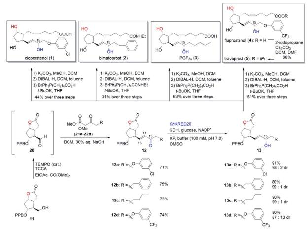
Fig. 5 Completion of the chemoenzymatic total synthesis of cloprostenol (1), bimatoprost (2), PGF<sub>2α</sub> (3), fluprostenol (4), and travoprost (5).
