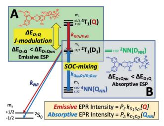
Fig. 5 (A) The reversed quartet mechanism (RQM). Mixing of chromophoric  ${}^2T_1$  and  ${}^4T_1$  states, mediated by conformational  $J_{\text{SQ-NN}^-}$  modulation, gives rise to emissive ESP for **6-Me-mPh-Pt**. (B) Spinorbit induced mixing of chromophoric  ${}^2T_1$  and the NN-based quartet state,  ${}^4\text{NN}$ , gives rise to absorptive ESP for mPh-Pt. The  ${}^2\text{NN}$  state can be observed spectroscopically (see ESI†).
