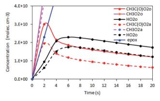
Fig. 3 Examples of simulations of the  $RO_2$  + alkene reactions, showing the concentration profiles in the reactor for RO<sub>2</sub> (red and pink), HO<sub>2</sub> (black), and epoxy products (blue). The solid lines are the profiles in the absence of alkenes and the dashed ones in the presence of alkenes. Top: CH<sub>3</sub>O<sub>2</sub> + isoprene reaction (experiment Alk05); bottom: CH<sub>3</sub>C(O)  $O_2$  + isoprene reaction (experiment Alk31).
