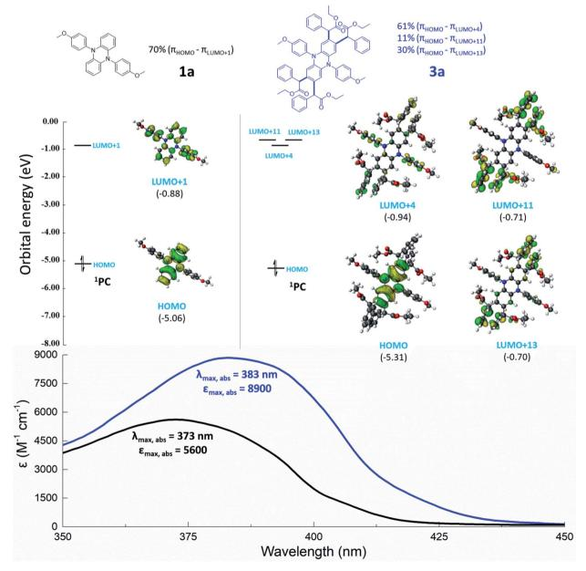
Fig. 6 TD-DFT calculations of orbitals and UV-Vis spectra of  ${\bf 1a}$  and  ${\bf 3a}$ . (Top) TD-DFT calculations and computationally predicted percentage contribution of orbitals involved in the photoexcitation of  ${\bf 1a}$  and  ${\bf 3a}$  at their corresponding  $\lambda_{\rm max,abs}$ . (Bottom) UV-Vis spectra of  ${\bf 1a}$  and  ${\bf 3a}$  acquired in DMAc.
