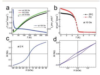
Fig. 3 Magnetic properties of TMCM–CrCl $_3$ . (a) Temperature dependence of the magnetic susceptibility ( $\chi T$ ). (b) Zero-field-cooling and field-cooling magnetization (M) under 10 Oe fields. (c) Field-dependent isothermal magnetization (M) at 2 K. (d) The zoomed views of magnetic hysteresis from (c).
