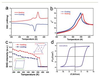
Fig. 2 Physical properties of TMCM–CrCl<sub>3</sub>. (a) DSC curves in heating and cooling runs. (b) The real part ( $\varepsilon$ ') of dielectric permittivity as a function of temperature. (c) Temperature-dependent SHG response in the heating and cooling runs. (d) P–E hysteresis loop measured along the polar axis of LTP at 373 K and 50 Hz.
