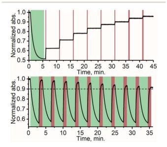
Fig. 4 Stepwise photoisomerization (above) of TFA by exciting PdNP with 10 s (last two were 20 s) doses of 740 nm excitation (dark red bars) in 5 min intervals. Cyclic photoswitching (below) of TFA/PdNP with 10 cycles of alternating 525 nm (direct excitation of *E*-TFA, green sections) and 740 nm (excitation of PdNP, dark red sections) excitation wavelengths.
