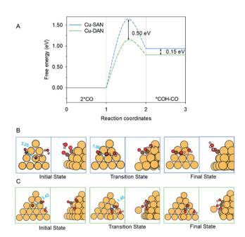
Fig. 3 (A) Reaction energetics involved in 2 \*CO dimerization and reduction to \*COH-CO at 0 V vs. RHE. Structures of the initial, transition and final states in CO-CO coupling on (B) Cu-SAN and (C) Cu-DAN, respectively. Minimum energy path for reaction barriers in panel A is found in Fig. S3.† Color code: Cu, orange; C, brown; O, red; H, pink. Distances are in Å.
