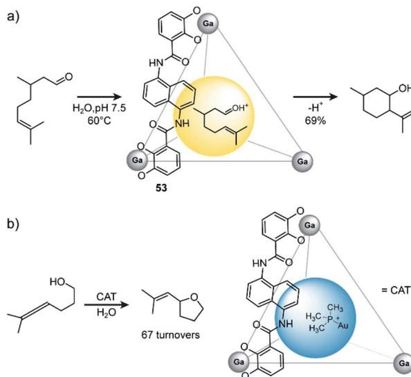
Fig. 24 (a) Prins cyclisation of citronellal catalysed by Raymond's  $Ga^{III}$  coordination cage. (b) Encapsulated catalyst  $Me_3PAu^+$  catalyses hydroxyalkylation of alcohol-tethered allenes. Reproduced from ref. 137 with permission from the Royal Society of Chemistry, copyright 2021.
