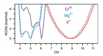
Fig. 4 Free energy as a function of coordination number of  $Cr^{3+}$ ,  $Mg^{2+}$ , and  $K^+$ . Solid and dashed lines indicate the KCl $-MgCl_2$  salt mixtures with and without  $Cr^{3+}$ , respectively.
