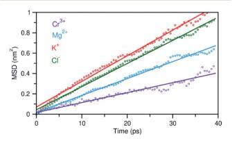
Fig. 6 Mean square displacement (MSD) of ions as a function of time, indicating faster dynamics in the order:  $K^+ > Cl^- > Mg^{2+} > Cr^{3+}$ . Dots represent the MSD data and solid lines are linear fits.
